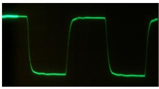
Frequency response at 1 W output into  $8\Omega$
