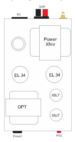
The Super Stealth + is designed to run the EL34 output tubes in self biasing mode (cathode bias), so no bias adjustments are required when changing tubes or powering up for the first time. The combined screen and plate current is around 58 mA per tube with a plate voltage of around 380 V. This results in a total dissipation of 21 W, well within the specifications of the EL34.
